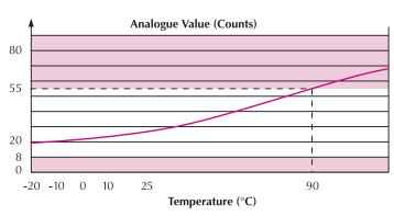
Fig.13 Typical response charateristic - XP95 Standard heat detector
